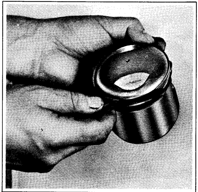
Figure 3-13. Measuring Ring Side Clearance
