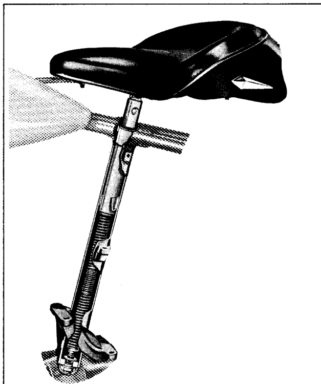
Figure 2-46. Cutaway of Seat Post Springing
