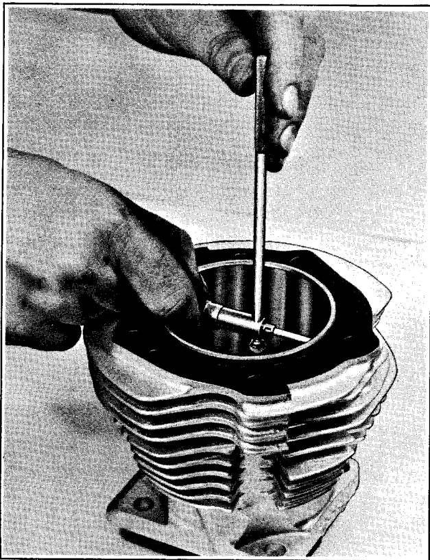
Figure 3-11. Measuring Cylinder Bore
