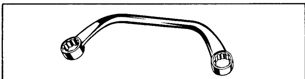
Figure 3-69. 94585-30 Cylinder Base Nut Wrench (5/8'')
