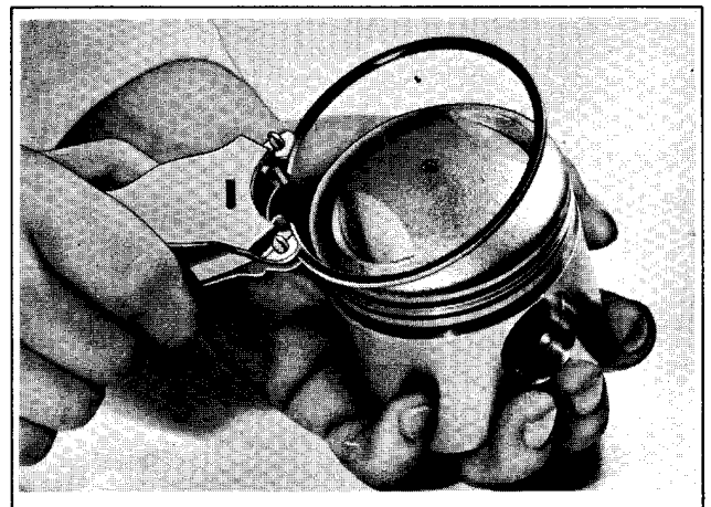
Figure 3-15. Assembling Rings with Ring Expander
