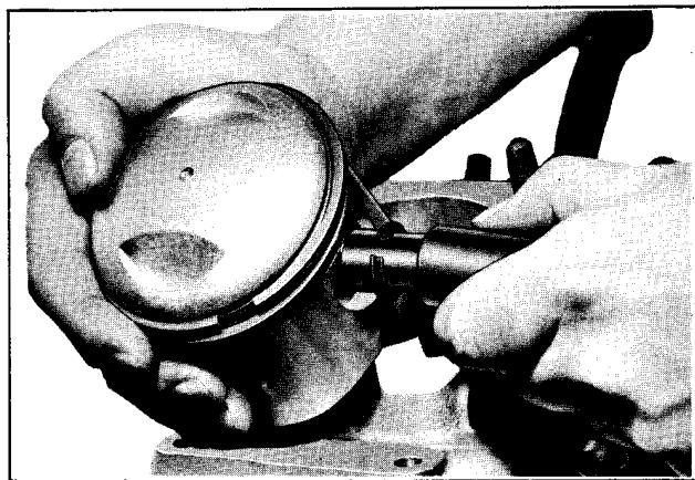
Figure 3-20. Inserting Piston Pin Lock Ring
